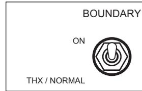
**Boundary Compensation** Use this switch to adjust the lower frequency output of the speaker to compensate for the typical sound colorations caused by placing the speaker close to a TV screen or building it into a wall unit or cabinet. To set these controls, sit in the prime listening position and have someone switch between the compensation choices, using well recorded dialogue or musical instrument recordings. Choose whichever switch position sounds most natural and real to you.
