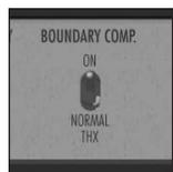
Large room boundaries, such as floors, walls, and ceilings, reinforce sound by acting essentially as acoustic “mirrors.” When the speaker is mounted too close to the corner or a wall/ceiling intersection, this sonic “reinforcement” often results in an unnatural heaviness or coloration of the sound.
