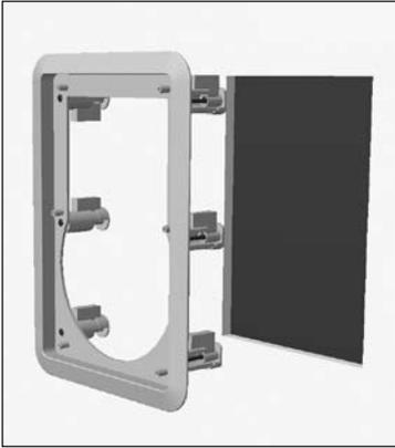
The clamping mechanism allows the wall material to range from ½ to 1½ inches (13 to 38 mm) in thickness. There must be a minimum depth behind the wall face of 3 5/8" (92 mm). As noted above, be sure to keep the edges of the cut-out at least ½ inch (13 mm) away from any stud or obstruction, as the rotating clamps will not operate properly if you don't. Insert the frame into the cutout and using a level or square carefully align it
