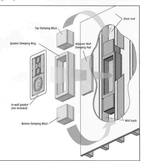
InWall Damping Kit Exploded View
