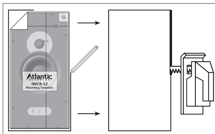
After determining the best location for the speaker as outlined above, use the enclosed template to cut the proper size hole.
