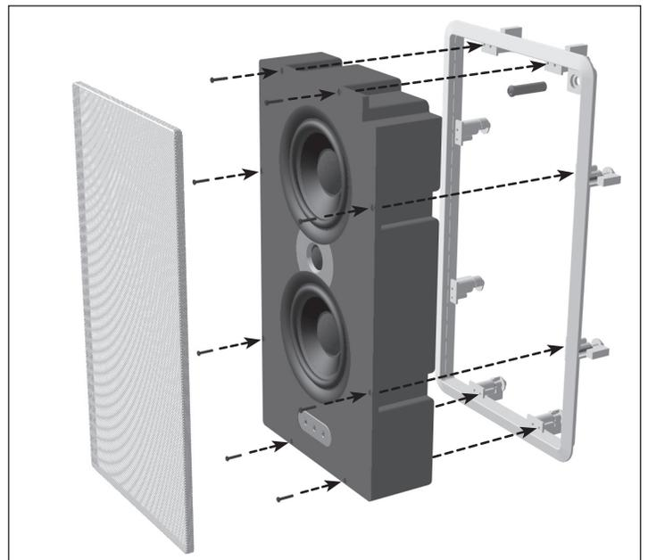
Once the frame is mounted in the wall, the speaker enclosure simply fits into the frame. Note that there is a foam anti-vibration pad affixed to the rear panel of the enclosure. This pad will eliminate any slight vibrations that occur if the back of the speaker enclosure contacts the wallboard in the wall cavity. Due to the usual slight dimensional variances in home construction, the IWCB either may or may not contact the wall surface behind it.
