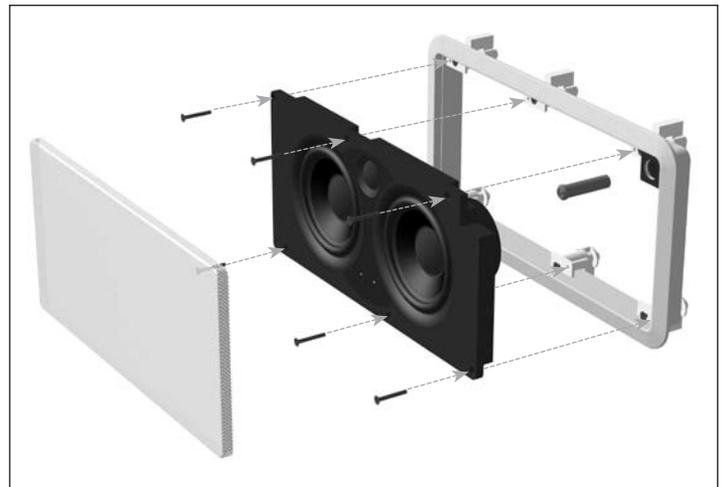
Once the frame is mounted in the wall, the speaker simply fits into the frame. Note that there is a gasket around the edge of the MDF baffle. This gasket ensures an airtight fit between the baffle and the frame. Therefore, the baffle may fit tightly in the frame. This is normal.
