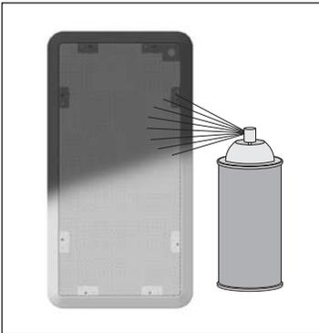
The white plastic frame and the metal grille may be left as is, or painted to match your décor. You can paint the frame before or after it is installed in the wall. Spray painting (using slightly thinned paint) is the best method to use for painting the grille. Before painting the grille, carefully peel off the cloth scrim. After painting the grille, use air pressure to "blow out" any grille holes that are filled in with paint.
