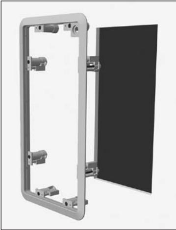
The clamping mechanism allows the wall material to range from ½ to 1½ inches (13 to 38 mm) in thickness. There must be a minimum depth behind the wall face of 3 ⅝" (92 mm). As noted above, be sure to keep the edges of the cutout at least ½ inch (13 mm) away from any stud or obstruction, as the rotating clamps will not operate properly if you don't. Insert the frame into the cutout and using a level or square carefully align it so it is level. Tighten the mounting screws, which will
