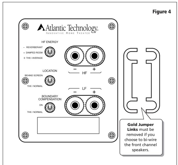
You can Bi-Wire by connecting two sets of speaker wires from the amplifier terminals to the input terminals on the back of the speaker enclosure. The wires should be attached to a single output terminal set on the amplifier. The other end is attached to the two sets of input terminals on the rear panel of the loudspeaker. Some manufactured Bi-Wire cables have only a single set of connectors at the amplifier end and two sets of connectors at the speaker end.
