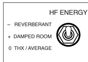
**High Frequency Energy** This control changes the tilt or roll-off slope of the tweeter. It has been designed to help compensate for different room acoustics. The THX/ Average position is intended for rooms with a reasonable combination of reflective (hard) and absorptive (soft) surfaces.
