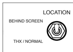
**Location** This control "shelves up" the upper midrange and high frequency energy from the speaker in the position marked Behind Screen. This is to compensate for the reduction of these frequencies when they are partially blocked by the materials in front of them if the speakers
