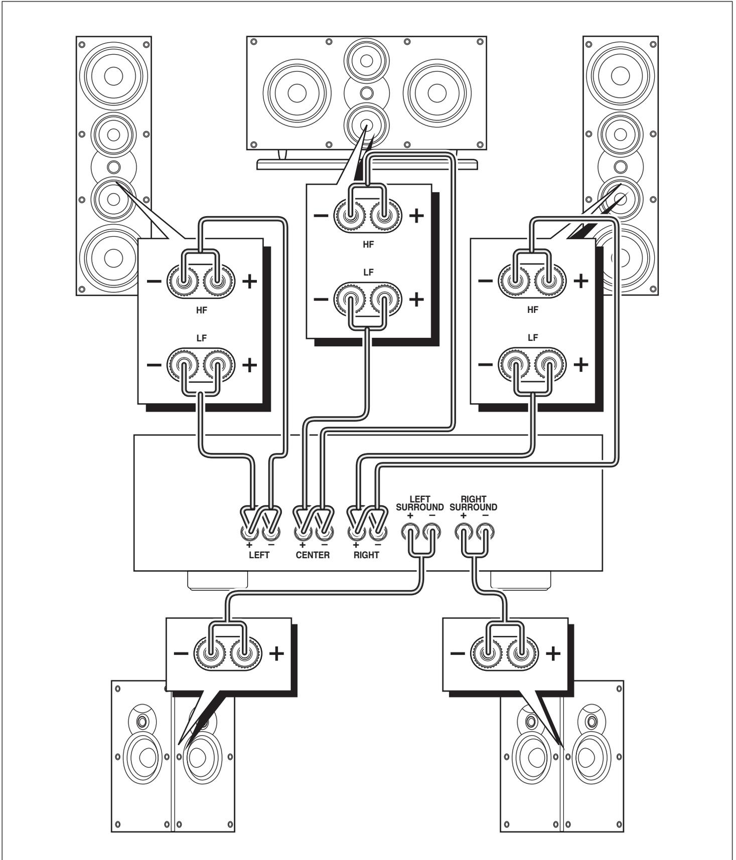
The terminals themselves are designed to allow the use of very heavy speaker wire or connectors. Be sure to tighten them securely, but don't over-tighten them.
