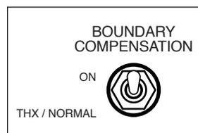
**Boundary Compensation** Use this switch to adjust the lower midrange output of the speaker to compensate for the typical sound colorations caused by placing the speaker close to a TV screen or building it into a wall unit or cabinet.
