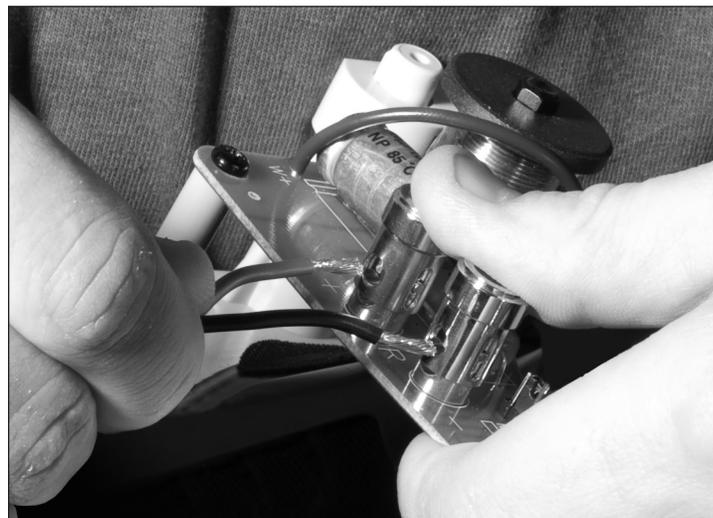
Strip about 1/2" (13 mm) of insulation from the connecting wires. Connect them to the appropriate push terminal, being careful to observe polarity (positive to the red terminal, negative to the black terminal).
