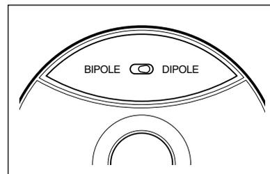
In Dipole mode the 4200 SR's produce ambience with minimal localization (best for most movies and video soundtracks), and more localizable sound in the Bipole mode (preferred for some music recordings). Switching between Dipole and
