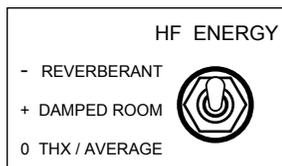
**High Frequency Energy** This control changes the tilt or roll-off slope of the tweeter. It has been designed to help compensate for different room acoustics. The THX/ Average position is intended for rooms with a reasonable combination of
