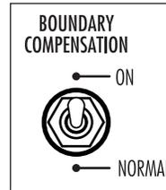
**Boundary Compensation** Use this switch to adjust the lower frequency output of the speaker to compensate for the typical sound colorations caused by placing the speaker close to a TV screen or building it into a wall unit or cabinet. To set these controls, sit in the prime listening position and have someone switch between the compensation choices, using well recorded dialogue or musical instrument recordings. Choose whichever switch position sounds most natural and real to you.
