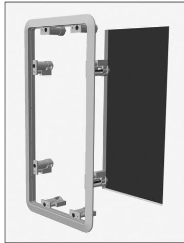
The clamping mechanism allows the wall material to range from 1/2 to 1 1/2 inches (13 to 38 mm) in thickness. There must be a minimum depth behind the wall face of 3 5/8" (92 mm). As noted above, be sure to keep the edges of the cutout at least 1/2 inch (13 mm) away from any stud or obstruction, as the rotating clamps will not operate properly if you don't. Insert the frame into the cutout and using a level or square carefully align it so it is level. Tighten the mounting screws, which will
