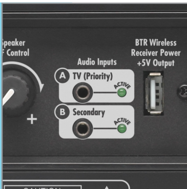
Priority Switching automatically selects the active input
