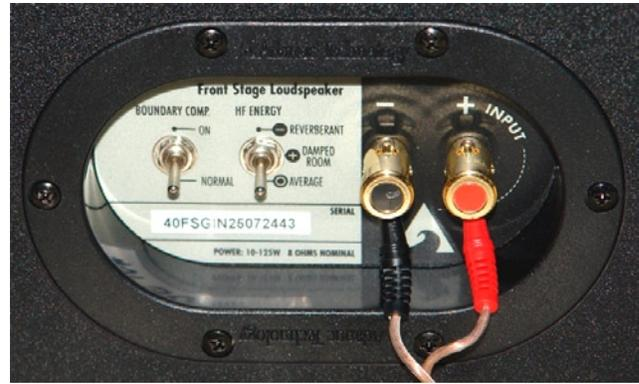
*Atlantic Technology FS-4000 Front Stage Flat Screen Speaker System - Connections and Adjustments Close-up*
