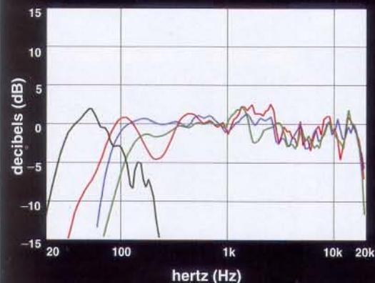
L/R 71 Hz to 17.7 kHz  $\pm 3.7$  dB    Surround 124 Hz to 17.1 kHz  $\pm 2.7$  dB
