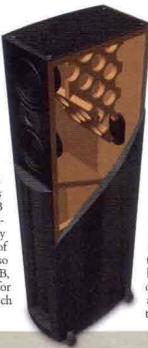
The AT-1's woofers are crossed over to its 1.1" silk-dome tweeter at 2kHz. the tweeter seeing a third-order slope and the woofer a secondorder handoff. While many two-way designs cross over at higher frequencies, the AT-1's 2kHz crossover ensures a more even dispersion pattern at the top of the woofers' passband and better integration with the tweeter. However, the lower the crossover frequency, the more energy a small tweeter is asked to produce, and the
