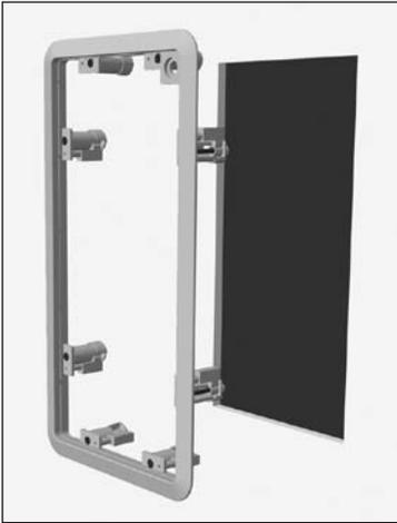
The clamping mechanism allows the wall material to range from ½ to 1½ inches (13 to 38 mm) in thickness. There must be a minimum depth behind the wall face of 3⅝" (92 mm). As noted above, be sure to keep the edges of the cutout at least 1½ inch (38 mm) away from any stud or obstruction, as the rotating clamps will not operate properly if you don't. The speaker assembly is designed to mount into the white frame, after the frame is mounted into the wall.
