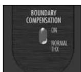
Large room boundaries, such as floors, walls, and ceilings, reinforce sound by acting essentially as acoustic “mirrors.” When the speaker is mounted too close to the corner or a wall/ceiling intersection, this sonic “reinforcement” often results in an unnatural heaviness or coloration of the sound.
