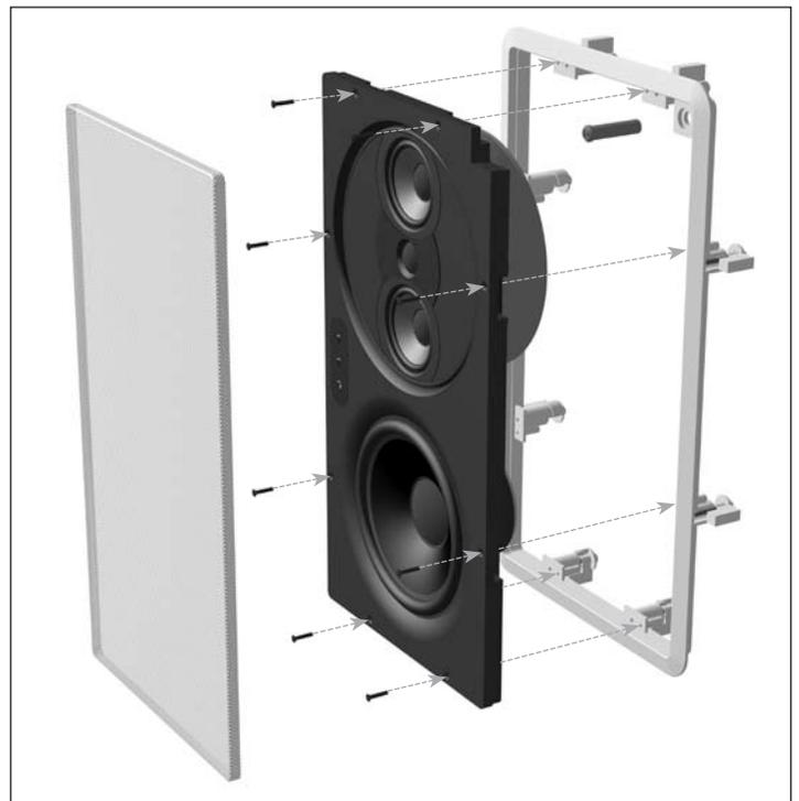
Once the frame is mounted in the wall, the speaker simply fits into the frame. Use the included screws to attach the Baffle to the mounting frame. *The baffle has a gasket around its outside edge to prevent unwanted air leaks, and may therefore fit tightly into the frame. This is normal.*
